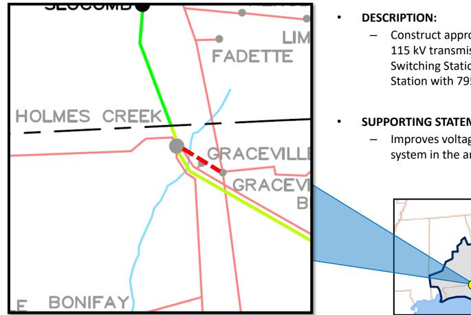
Construct approximately 1.08 miles of new 115 kV transmission line from Graceville Switching Station to FPL's Homes Creek Station with 795 ACSR at 100°C.
